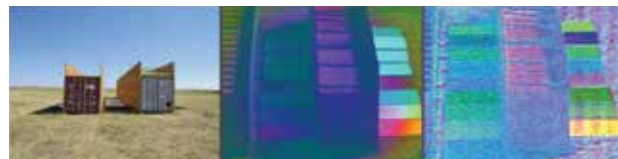
Figure 18: (Left) Indirect illumination site; (Middle) 3-band Mid-Wave Infra-Red (MWIR) image; (Right) Composite image using three principal components of the thermal hyperspectral image.
