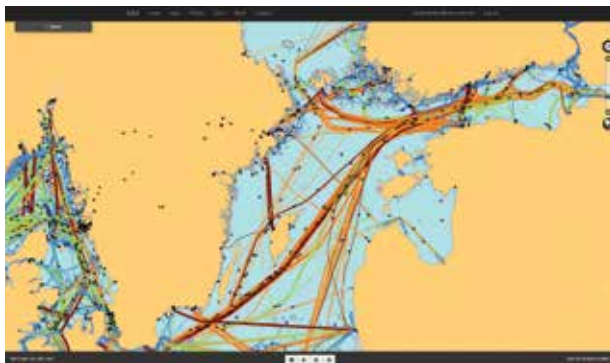
Figure 33: Real-time AIS traffic on top of the recognised traffic schemes in the area of operations at CWIX 2015. The TREAD methodology generated the patterns of life, which are colour-coded depending on the average velocity of vessels on the route.
