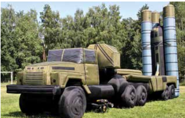
Figure 49: Representative deception technique using inflatable systems.
